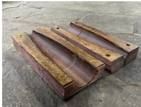
Figure 5 Split-Pattern Female Coupler Mould
