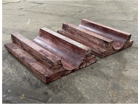
Figure 11 Split-Pattern Female Coupler Mould
