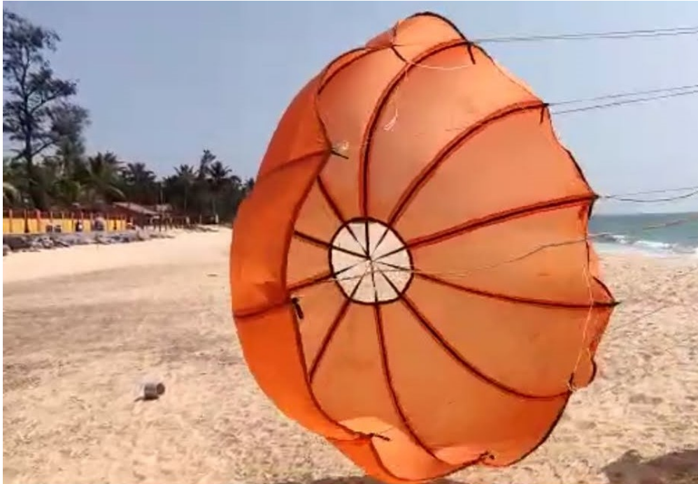
Figure 61 The parachute fully expanding after reefing lines are cut
