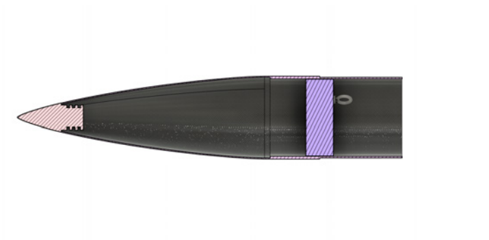
Figure 8 Sectional View of Nosecone with nose tip
