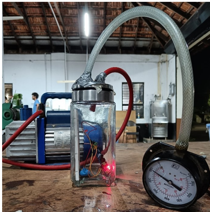
Figure 62 The vacuum pump used to test the apogee detection algorithm.
